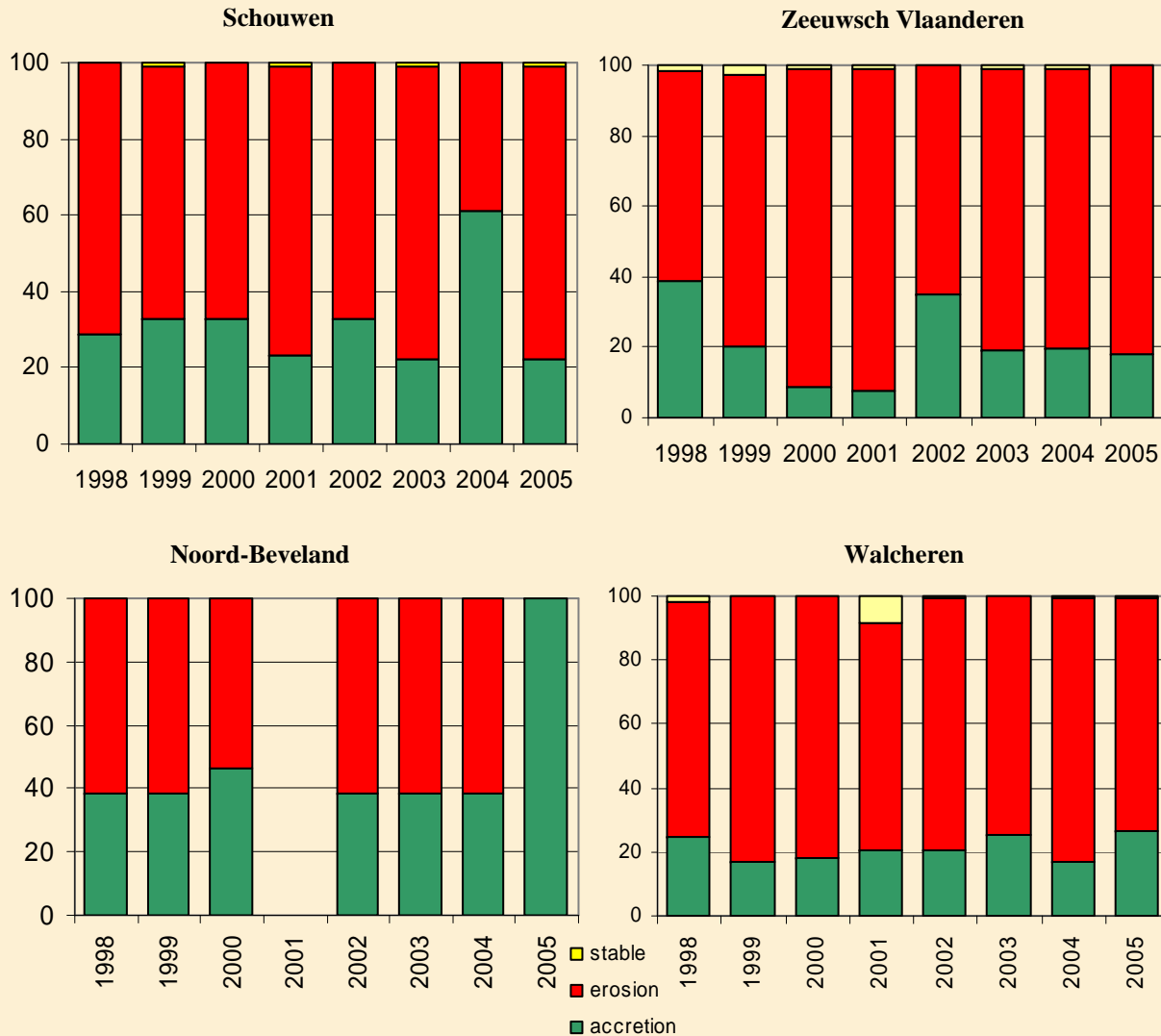
Percent of the coastline that is eroding, accreting or stable Zeeland coastal management units (RWS/RIKZ 2005)
